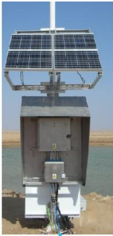
Solar powered surface interrogator radios data to Muscat HQ
