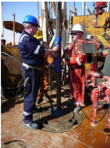
SmartCell® attachment to tubing string
