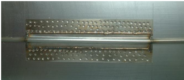
SmartWeld spot welded to steel structure
