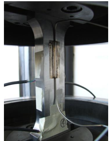
SmartWeld undergoing calibration and fatigue testing at UKAS accredited testhouse
