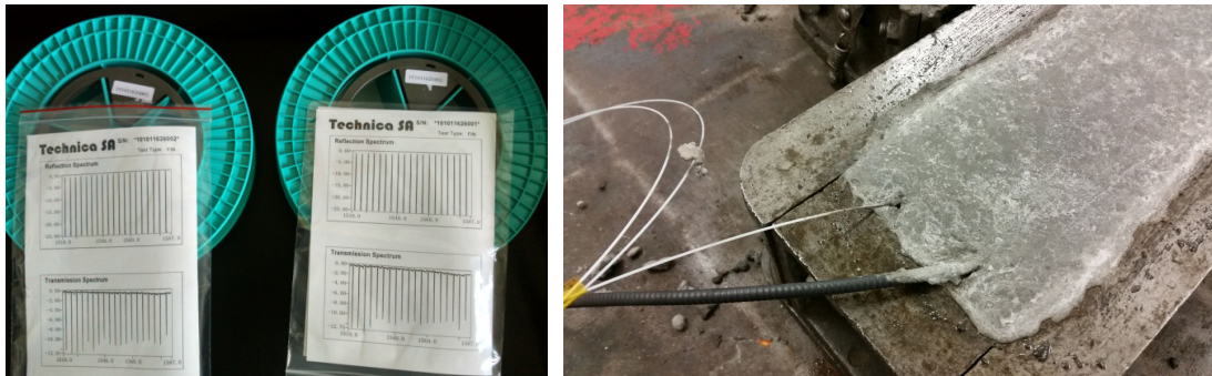
Highlights of representative figures inside this article: GFRP-FBG Spools before and after deployment
