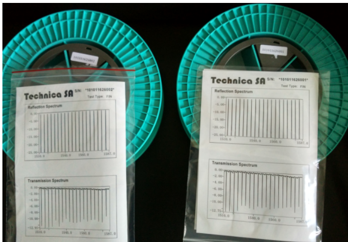
Fig.5. T130 GFRP FBG cable sensors ready for field deployment.
