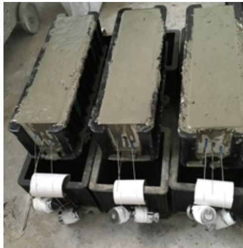
Fig.9. T130 sensing cables buried in concrete ready for measurements
