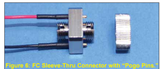
Figure 5: FC Sleeve-Thru Connector with "Pogo Pins."
