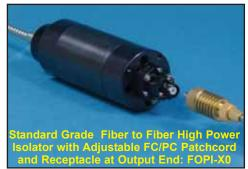
Polarization insensitive isolators use birefringent crystals to separate the input beam into two orthogonal polarizations, transmit them through the faraday crystal and then recombine them to produce an output beam.
