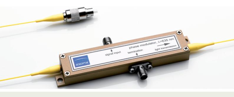
The Integrated Optical Phase Modulator is a compact fibercoupled electro-optical modulator that works based on MgO:LiNbO<sub>3</sub> and LiNbO<sub>3</sub> crystals. Providing fast electrooptical response, it allows phase modulation with frequencies as high as the Gigahertz range. Available modulators can handle wavelengths in the visible and the infrared spectral range.
