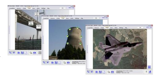
The ENLIGHT Sensing Analysis Software tool is included with the sm125 and sm130 Optical Sensing Interrogators. It is also available pre-loaded on the Micron Optics sp125 or sp130 sensor processing units which interface directly with sm125 or sm130 Optical Sensing Interrogators. ENLIGHT is a standard feature on other Micron Optics interrogators such as the si225, si230, si725 and si730.
