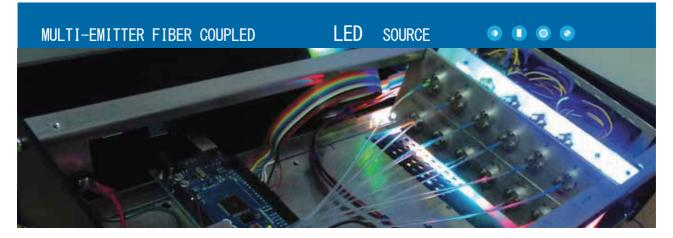
Our multi-emitter fiber coupled LED light sources are built on a modular LED platform that is configurable to the customer's required spectral distribution. An integrated light mixing module ensures both spectral and spatial uniformity at the the output aperture of a 5 mm diameter fiber optic bundle. The initial configuration spans the entire visible spectralng a selection doscrete single wavelength emitters combined with high power white LEDs.
