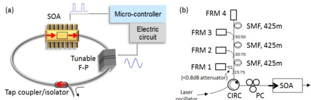
Figure 4. Simplified SCFP ring laser architecture and buffer-multiplier network
