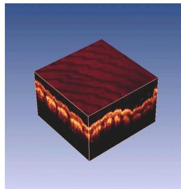
Figure 3. Human Finger imaged at 232,000 scans/second with FFP-TF based FDML laser.
