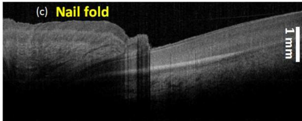
Figure 6. Artifact-free OCT image taken with 100kHz SFCF laser.
