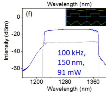
Figure 5. Spectral characterization of SCFP ring laser
