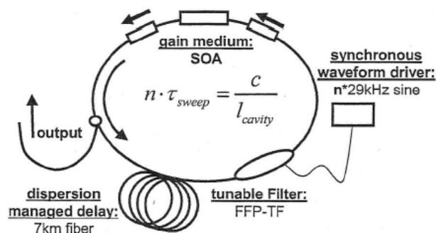
Figure 2. Simple FDML ring architecture employing an FFP-TF
