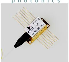
with an internal thermistor, TEC, and photodiode. Axcel's trademark laser chip design creates un-measurable degradation free and long lifetimes that make our chips among the most reliable in the industry today. The 500 mW output power has a Lambda-Lok option available for increased wavelength stability at  $\pm 0.5 \text{nm}$ . Our 808nm multi mode line serves a broad range of applications including solid state pumping, laser display, graphics, medical, dental, industrial, and defense.
