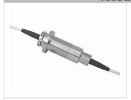
The MJP series FORJs are uniquely designed to distinguish themselves from other Princetel single-channel FORJs such as the the popular RPT model. Unlike model RPT, MJP is not fluid filled. It offers higher return loss performance (>55 dB). Start up torque is much lower. It can also accept custom fibers, primarily fibers with cladding diameter larger than 125 um.
