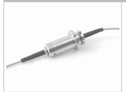
Model RPC series FORJs are designed to offer extreme pressure rating of 20,000 psi while maintaining identical optical performance as the RPT series. 900 um Hytrel tight buffer and 2.9 mm armored jacket are standard cable arrangements.
