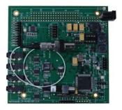
Highly integrated video/data multiplexers. Four channels of high-quality video and 6 channels of standard bidirectional data are multiplexed into one optical channel and transmitted through one standard fiber, single or multi mode. Ideal for robotic vehicles such as underwater ROVs (remotely operated vehicles).
