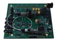
Video 4 (NTSC, PAL, Y/C, RGB: 10 bit/AD Data 6 (4xRS-232, 2xRS-485/422) Fiber 1 (SMF28, 50/125um, or 62.5/125um) λ 1310/1550 nm SM (850/1310 nm for MM)
