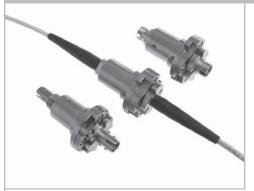
The R series Single-channel (SM or MM) rotary joints offer the most versatile designs on the market. The rugged body allows fiber pigtail, ST, or FC receptacles on either the rotor side or the stator side. One can configure the package to fit his need exactly. The standard base models are RPT, RFC, and RST for pigtails, FC/UPC, and ST/PC receptacles.
