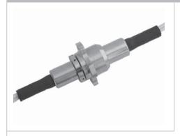
This dual-pass Fiber Optic Rotary Joint (FORJ) connects two independent fiber channels simultaneously. It allows uninterrupted transmission of optical signals while rotating along the common mechanical axis. It is designed to accommodate at least one multimode fiber. The other channel can be either single or multimode fiber. Princetel's unique design has raised the standard for size and performance of two-channel FORJs.
