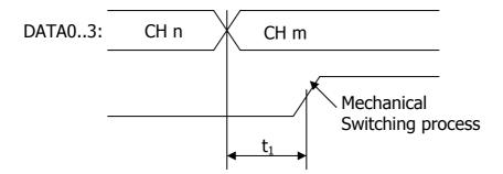
After detecting a new switching state (binary code) at the data input port, the switches moves to the corresponding channel after time delay  $t_1$ . In order to avoid problems this code must be kept constant for this period.
