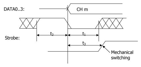
By a HIGH– LOW slope, data at the parallel interface ports are transferred into the switch and stored there (latch). The LOW level for the strobe input must be constant for a time period  $t_1$ . Before the HIGH – LOW slope the strobe signal has to be at HIGH level at least for a time duration  $t_2$ . Switching occures after a duration  $t_3$ .
